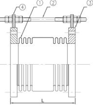
Model - SSEJ-500N/500H - WITHOUT TIE RODS Model - SSEJ-500N-SG / 500H-SG -WITH OPTIONAL TIE RODS FLANGED ENDS - ANSI ASA-150/ 300 OR BS4504 PN16 /PN25/PN40
