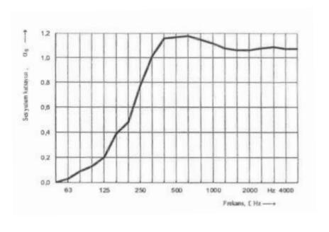
Due to ISO 11654 standard, weighted sound absorption coefficient is;
