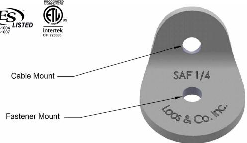
The SAF-1/4 is designed for use in attaching seismic cable bracing to steel structural members. The limitations of use are governed by the fastener diameter as a 1/4 inch (6mm) fastener is only listed for use with steel, as per NFPA-13. Will accept both metric and imperial fasteners. The cable mount will accept Gold, Orange, or Green cable.
