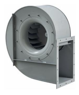
Engineered for durability, this direct drive, single inlet centrifugal fan is crafted from high-quality Mild steel, coated with a cataforesis primer and finished with an epoxy paint layer for superior protection. Built to perform in extreme conditions, it efficiently circulates air in temperatures ranging from -20°C to 100°C, ensuring reliable operation in continuous use.
