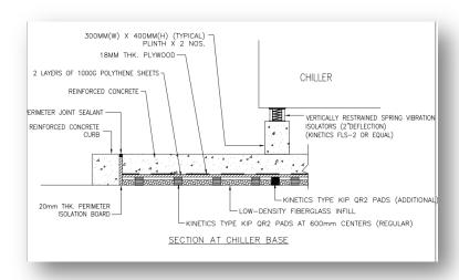
The Model KIP isolators can be spaced at intervals of 12, 16, or 24 inches on center, providing flexibility in their application. These isolators come in a variety of densities, allowing the system to accommodate a wide range of load conditions under a single slab, all while maintaining a consistent natural frequency. This flexibility ensures that the RIM system can be adapted to various project specifications, making it ideal for applications that demand precise noise control.
