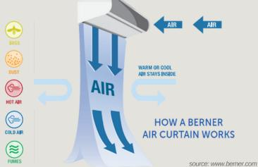
This stream acts as an invisible shield, preventing the infiltration of outside air, dust, insects, odours, and pollutants while allowing unobstructed passage for people and goods (1).
