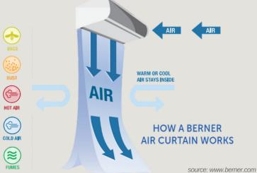
This stream acts as an invisible shield, preventing the infiltration of outside air, dust, insects, odours, and pollutants while allowing unobstructed passage for people and goods (1).
