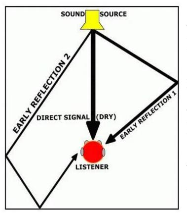
Reverberation, or "reverb" for short, is what you hear in a room when sound is produced. There's direct sound-the waves of sound in the air that go from the speaker to you directly-but the sound is propagated in a wave out in all directions from the source.
