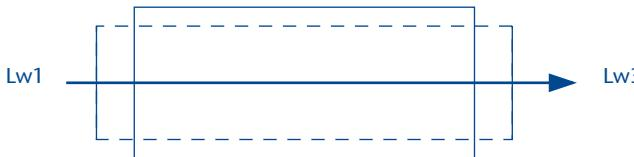
Attenuation is the difference between the acoustic capacity Lw1 in the test channel in front of the ducting and the acoustic capacity Lw3 in the test channel after the ducting (averaged over three measuring points).
